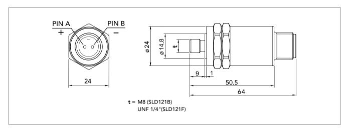
The vibration transducer SLD121B and SLD121F are piezoelectric accelerometers of compression type with built-in preamplifier, designed for vibration monitoring of industrial machinery. The electrical signal is isolated from the transducer housing.
