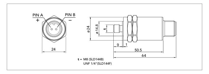
The vibration transducer SLD144B and SLD144F are piezoelectric accelerometers of compression type with built-in preamplifier, designed for vibration monitoring of industrial machinery. The electrical signal is isolated from the transducer housing.
