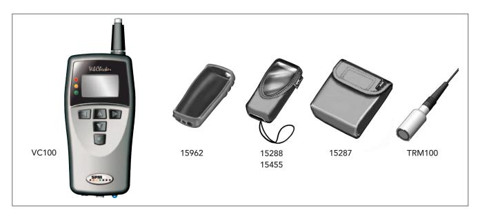
VibChecker is an instrument for fast and easy measurement of machine condition in preventive maintenance. The instrument and the monitoring technique are based on the recommendations of ISO 2372 and ISO 10816 standards for broad band measurements of vibration. These standards make the assumption that limited information, obtained easily and at a low cost, is often as useful as a detailed analysis using expensive equipment and elaborate techniques.
