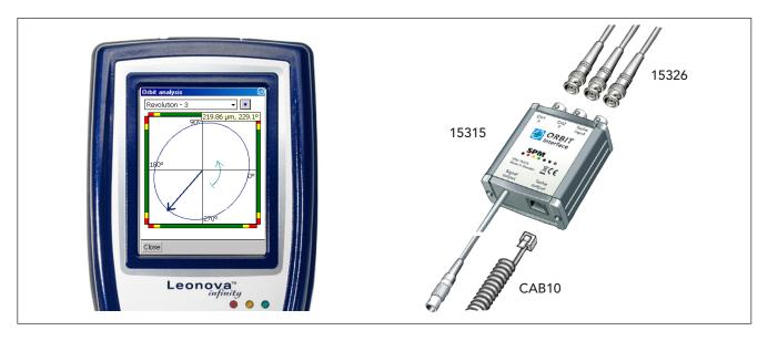
Orbit analysis is a vibration measurement function offered with Leonova infinity, for either unlimited (LEO138) or limited use (LEO238). The resulting orbit graph shows the movement of the shaft's centerline and is used to detect failures like rubs, unbalance, misalignment or oil whip on machinery with journal bearings.
