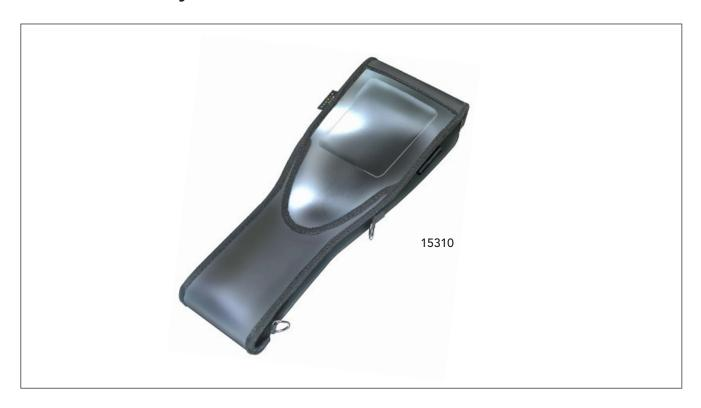
Protective cover 15310 is an optional accessory for the hand-held machine condition analyser Leonova™ Infinity. The cover, made of foamed polyester fabric, protects the instrument against shocks, splashes and dirt, IP65. The transparent plastic window makes Leonova easy to operate via the keypad and the touch screen. The cover is provided with holders for wrist strap and stylus.
